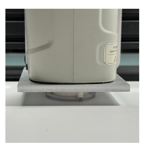
The operator can define both: "up" and "down" positions. That enables adjustment to materials of different thicknesses.
