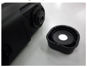
How to attach) Align the line of the main body and the line of the calibration cap (hereinafter, gray line) and rotate it in the direction of the arrow described on the calibration cap.
