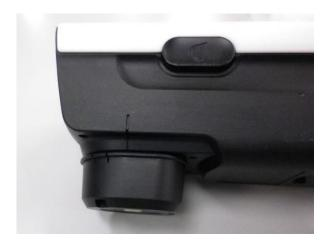
Reference) At the time of measurement, the calibration cap can be stored as shown below.
