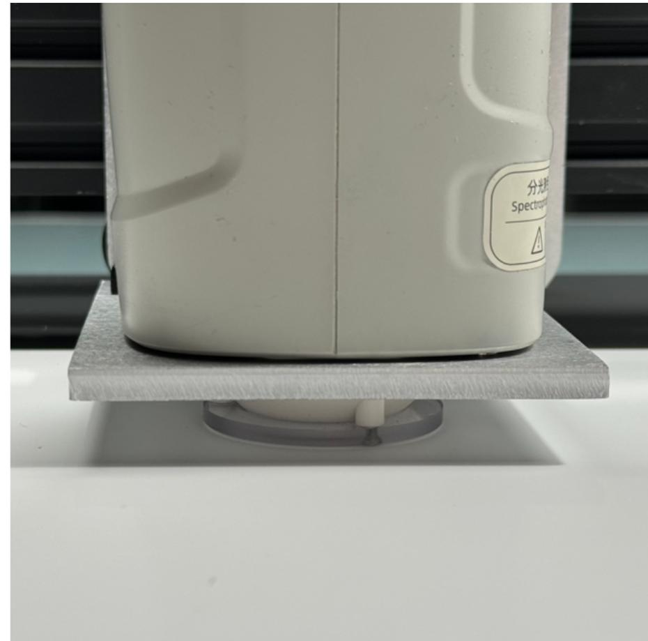
The operator can define both: “up” and “down” positions. That enables adjustment to materials of different thicknesses.
